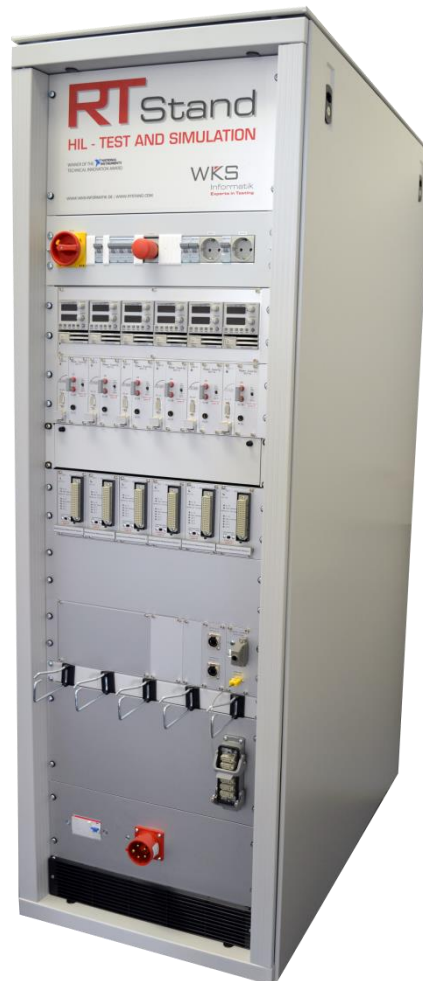
Gateway tester for 6 DUTs used for PV, DV and lifetime tests
