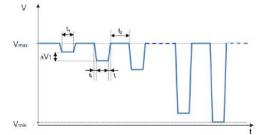
All relevant connections of the original circuitry must be tested. The DUT must be addressed in the same way as it is in the vehicle circuit. The test must be performed at various voltages between 0 V and the maximum values specified below:
