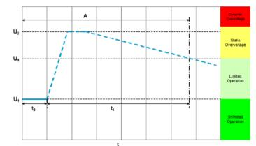
**Part 2** The DUT is connected to a powerful 4 quadrant amplifier and must be operated for at least t0 at U1. Thereafter, the activation of the feedback begins and at maximum regenerative current of the DUT, the decrease in the regenerative power abruptly (toff) must be terminated.
