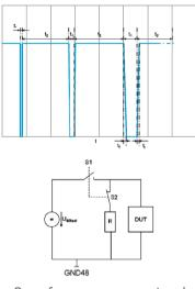
One reference measurement each with 1 k $\Omega$  (± 5%) and 10  $\Omega$  (± 5%) as a DUT substitute must be performed and documented.
